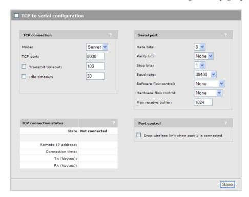
2. Select Network > TCP serial. The TCP to serial configuration page opens.
