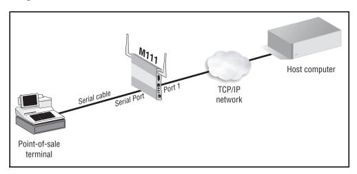
If you enable the **Drop wireless link when port 1 is connected** feature, the M111 can automatically switch between port 1 and the wireless link. See *Port control on page 3-26*.
