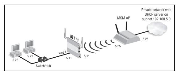
(Although this scenario shows two connected devices, up to 20 Ethernet devices can share the wireless link, with each device getting its own unique IP address from the DHCP server.)
