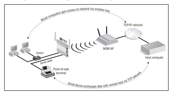
In this sample deployment, the M111 provides a wireless link to a TCP/IP network for a pair of desktop computers and a serial point-of-sale terminal. An MSM AP is used to create the wireless network.
