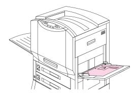
Place media into the input tray with the side to be printed on face up for single-sided printing (see figure 8). For letter- or A4-sized media, place the top of the page toward the rear of the printer and the long edge toward the printer. For media sizes larger than letter and A4, place the top (short) edge of the page toward the printer.
