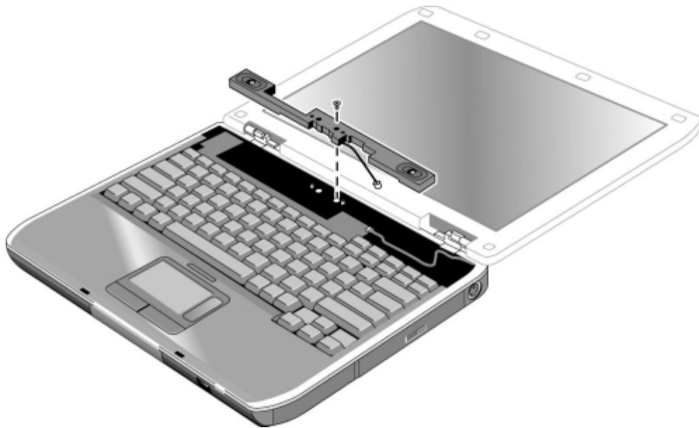
Figure 2-11. Removing the Speaker Assembly
