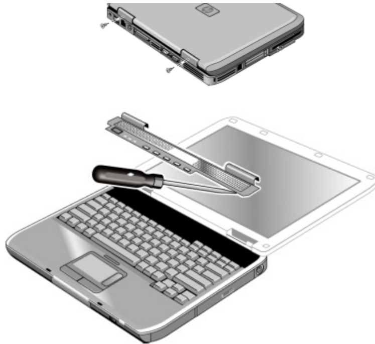
Figure 2-9. Removing the Keyboard Cover
