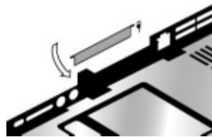
Figure 2-37. Removing a PCMCIA Door
