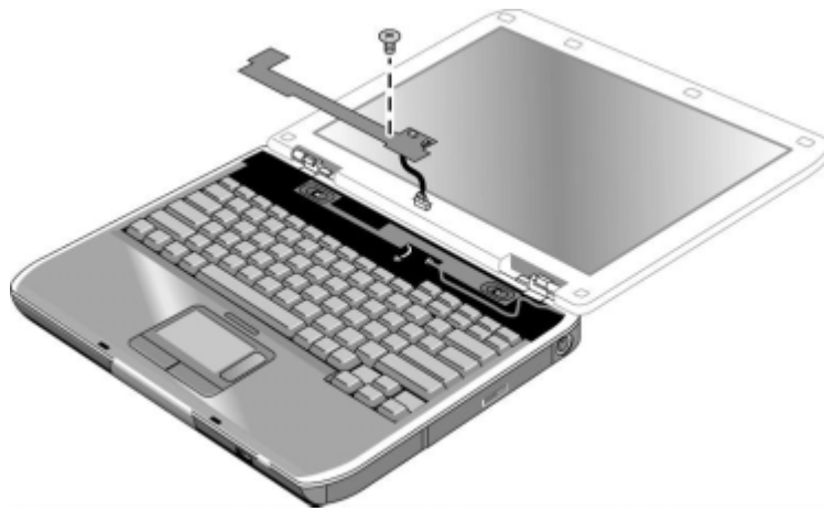
Figure 2-13. Removing the Switchboard PCA HP Pavilion 4300, 4200, and 4100, HP nx9005 and nx9000, Compaq Evo Notebook N1050 and 1010, and Compaq Presario 2100 and 1100 Models
