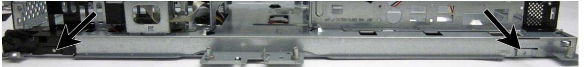
Figure 7-81 Display panel screw locations – 6300 models – CMI panel
