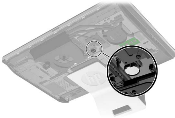
Figure 7-32 Locating the battery
