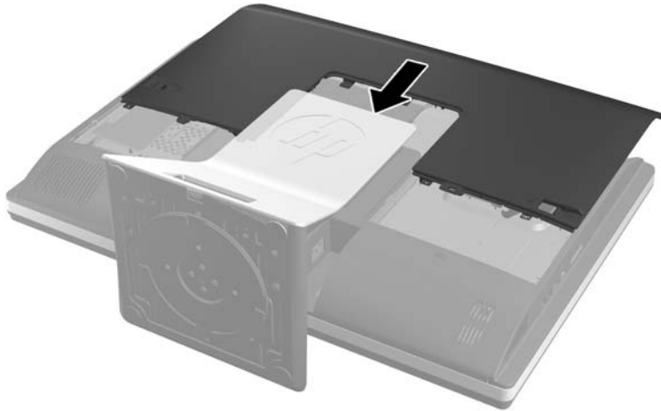
Figure 7-7 Replacing the access panel
