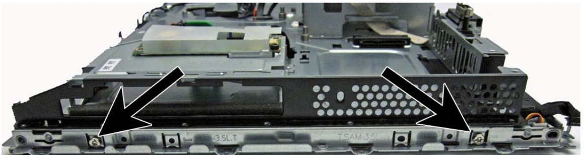
Figure 7-83 Display panel screw locations – 8300 models – CMI panel
