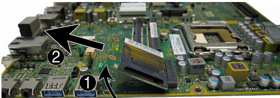
Figure 7-69 Removing the card reader board
