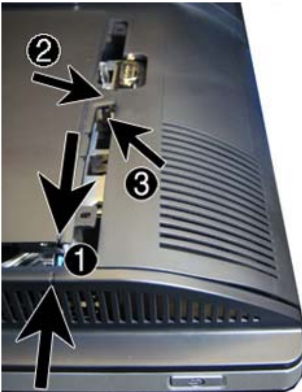
Figure 7-8 Access Panel Replacement
