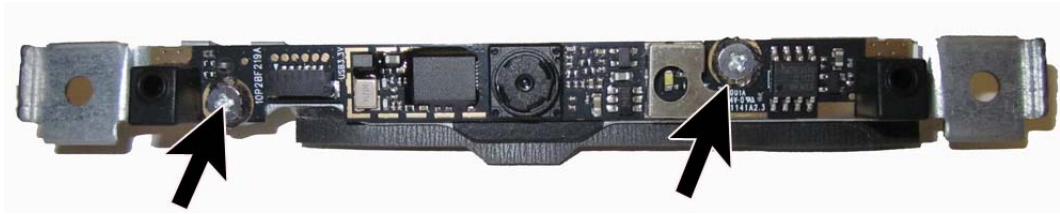
Figure 7-39 Disconnecting the webcam module cable
