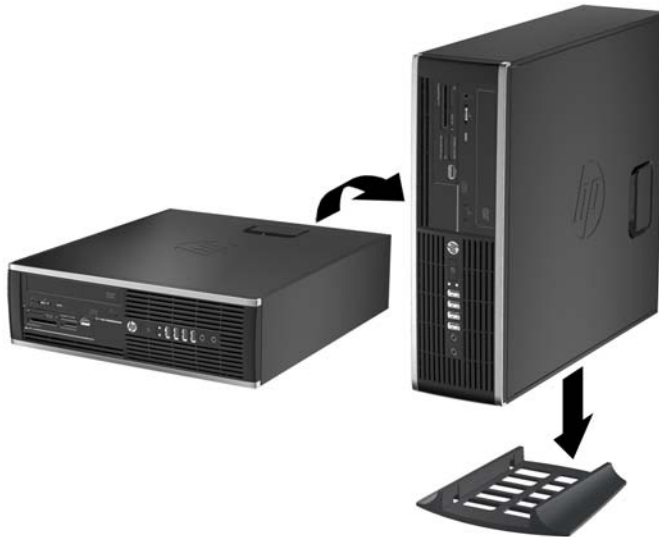
Figure 3-6 Changing from Desktop to Tower Orientation
