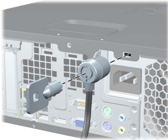
Figure 3-40 Installing a Cable Lock
