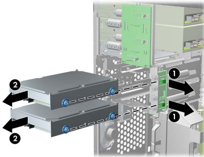
Figure 2-25 Removing a Hard Drive
