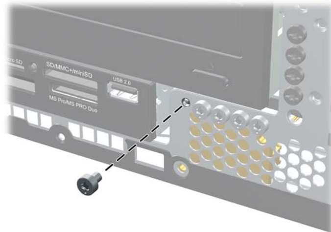
Figure 3-50 Retrieving the Front Bezel Security Screw
