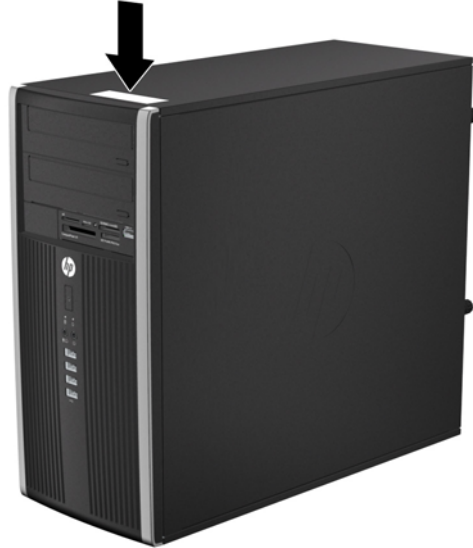
Figure 1-8 Microtower Serial Number and Product ID Location
