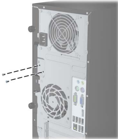
Figure C-1 Removing the Smart Cover Lock Screws from the Microtower
