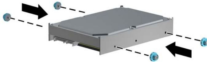
Figure 3-37 Installing Hard Drive Guide Screws
