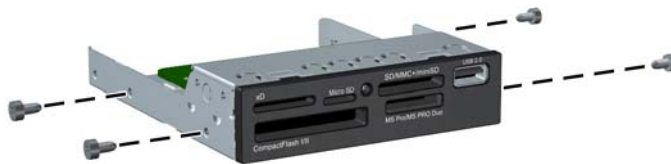
Figure 3-29 Installing Guide Screws (Media Card Reader Shown)
