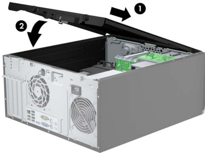
Figure 2-2 Replacing the Computer Access Panel
