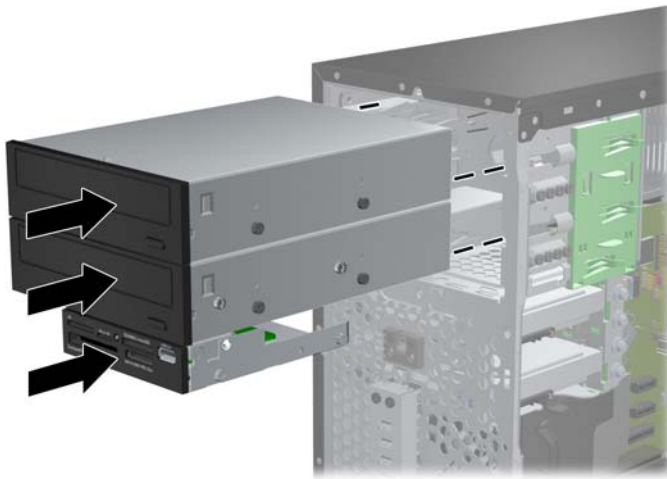
Figure 2-21 Sliding the Drives into the Drive Cage
