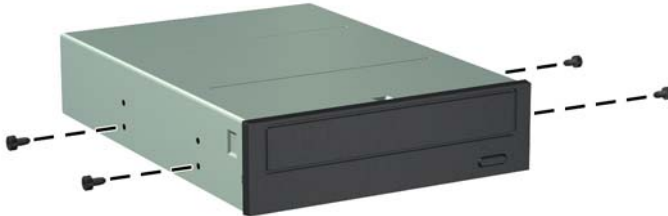
Figure 2-20 Installing Guide Screws (Optical Drive Shown)
