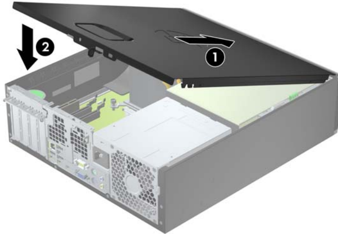
Figure 3-2 Replacing the Computer Access Panel
