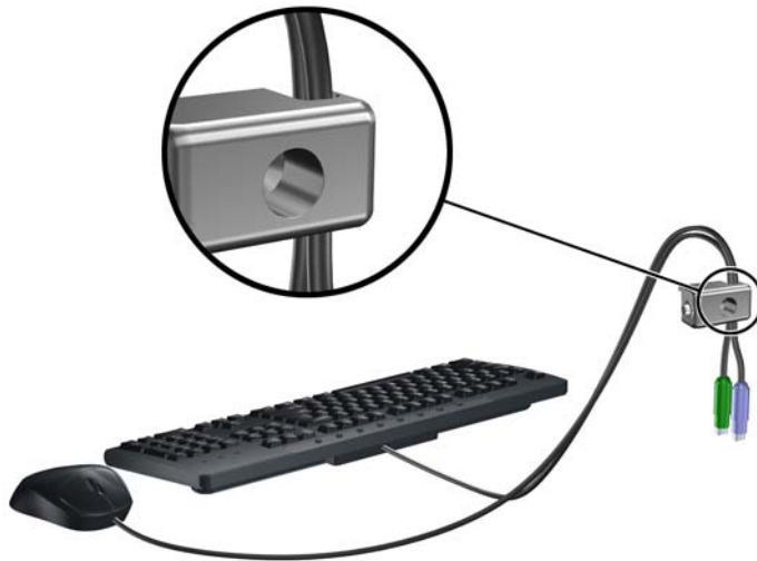
Figure 3-46 Threading the Keyboard and Mouse Cables
