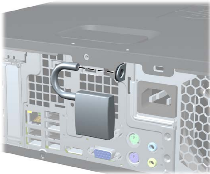
Figure 3-41 Installing a Padlock
