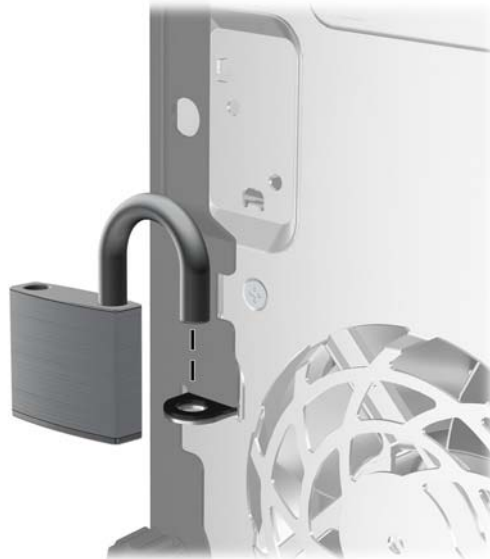
Figure 2-33 Installing a Padlock
