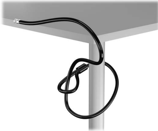
Figure 2-34 Securing the Cable to a Fixed Object
