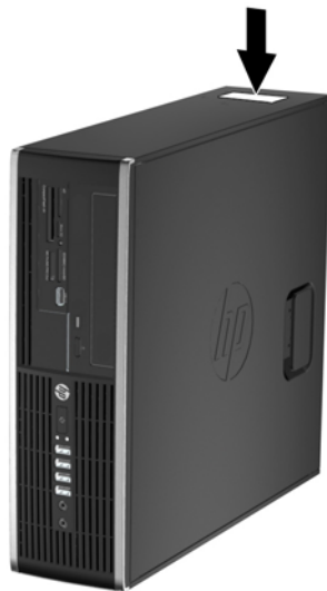
Figure 1-9 Small Form Factor Serial Number and Product ID Location
