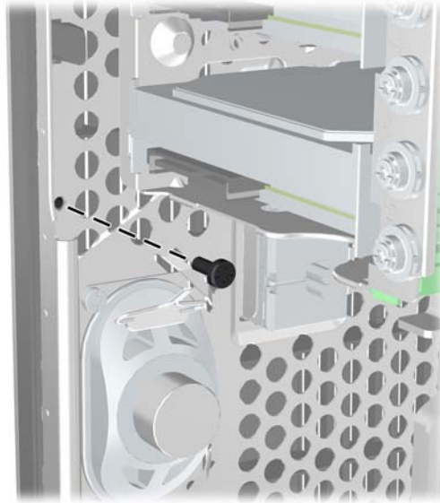
Figure 2-43 Installing the Front Bezel Security Screw
