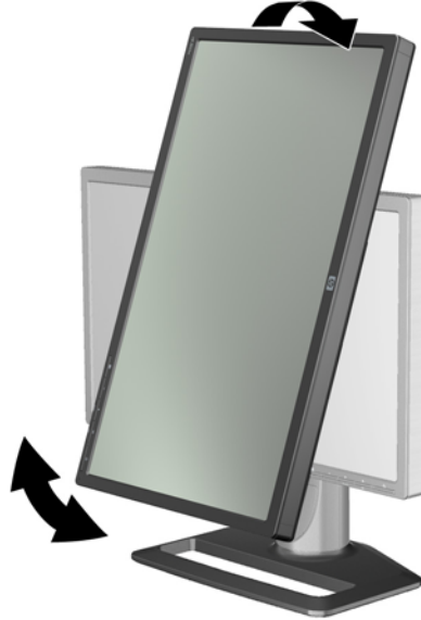
Figure 3-10 Pivoting the Monitor
