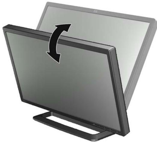
Figure 3-7 Tilting the Monitor
