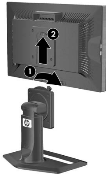
Figure 3-11 Removing the Monitor from the Pedestal Base
