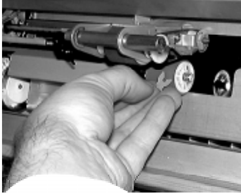
Figure 4-41 Removing Lower Roller Clip
