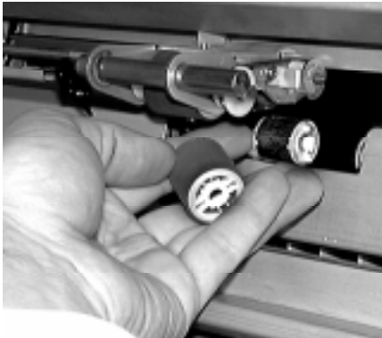
Figure 4-42 Removing Lower Rollers from Shaft
