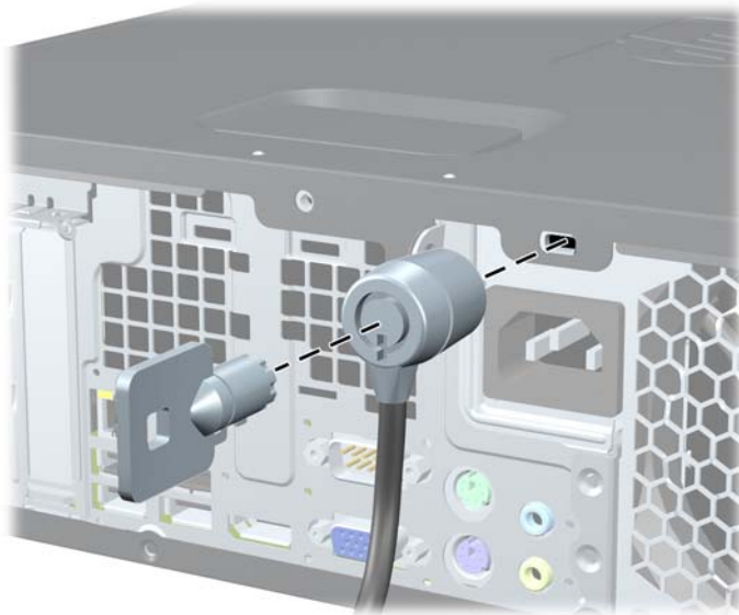
Figure 9-58 Installing a Cable Lock
