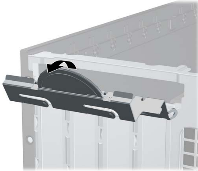
Figure 9-8 Opening the Expansion Slot Retainer
