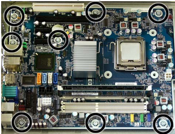
Figure 9-54 Removing the system board
