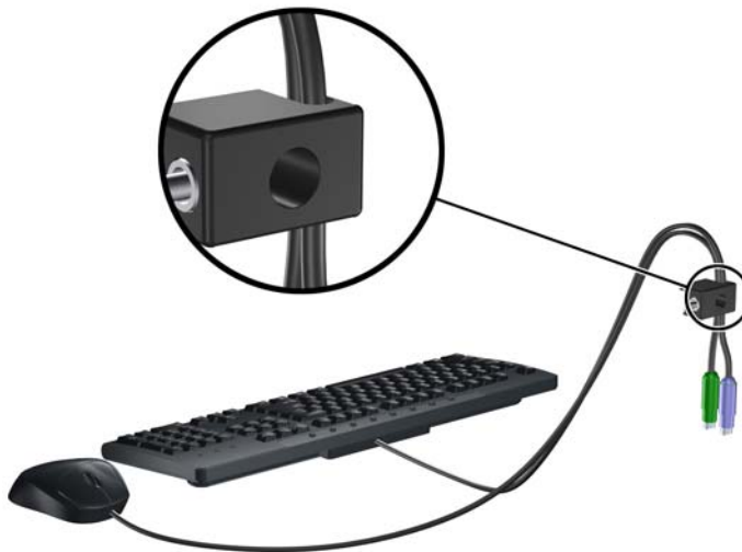
Figure 8-41 Threading the Keyboard and Mouse Cables
