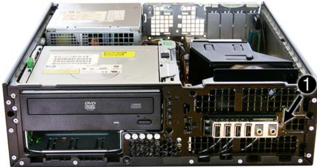
Figure 9-47 Removing the front I/O device/power switch
