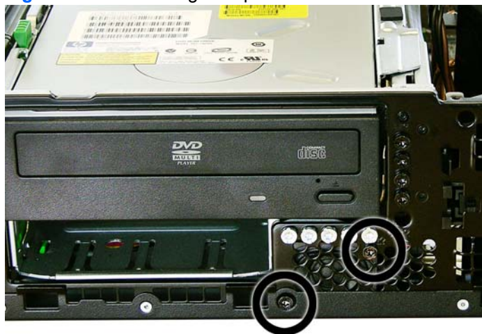
Figure 9-50 Removing the speaker
