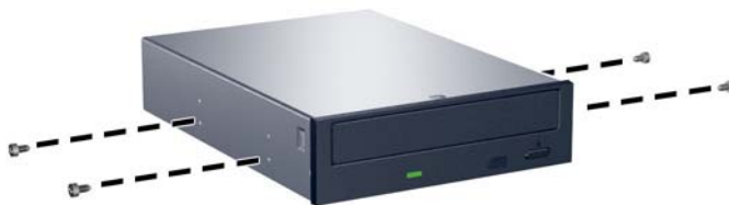
Figure 8-20 Installing Guide Screws (Optical Drive Shown)
