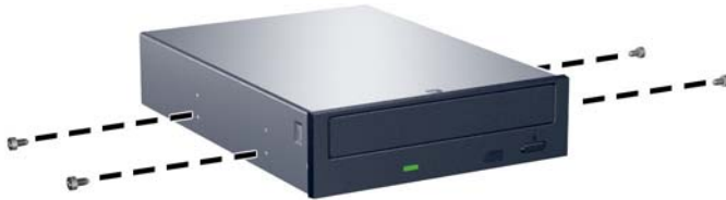
Figure 9-22 Installing Guide Screws in the Optical Drive
