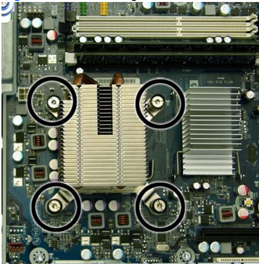
Figure 9-51 Removing the heat sink
