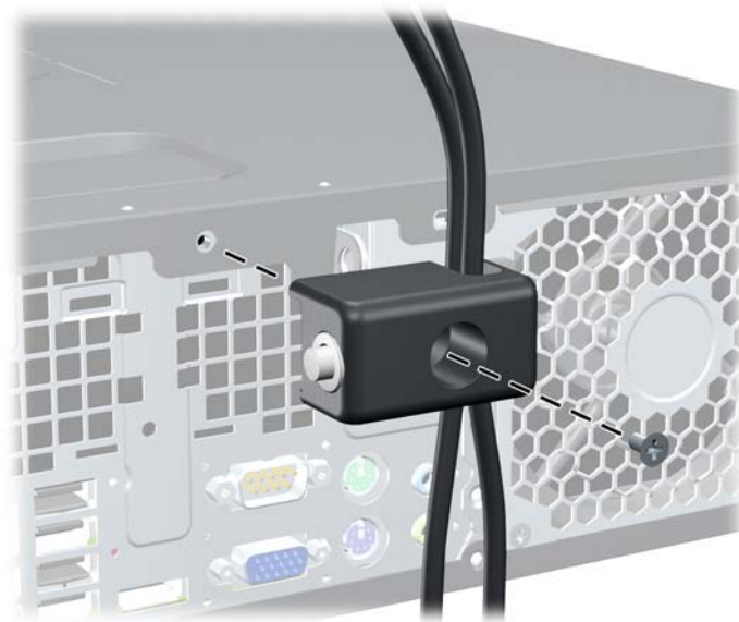
Figure 9-62 Attaching the Lock to the Chassis
