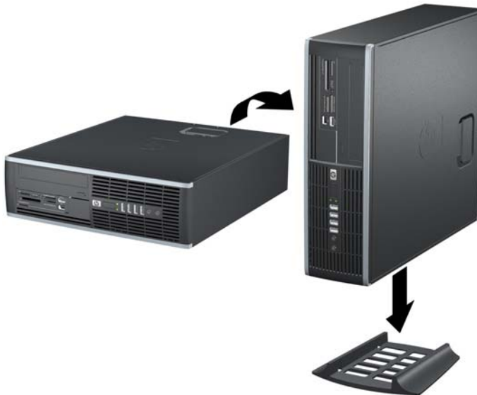
Figure 9-66 Changing from Desktop to Tower Orientation
