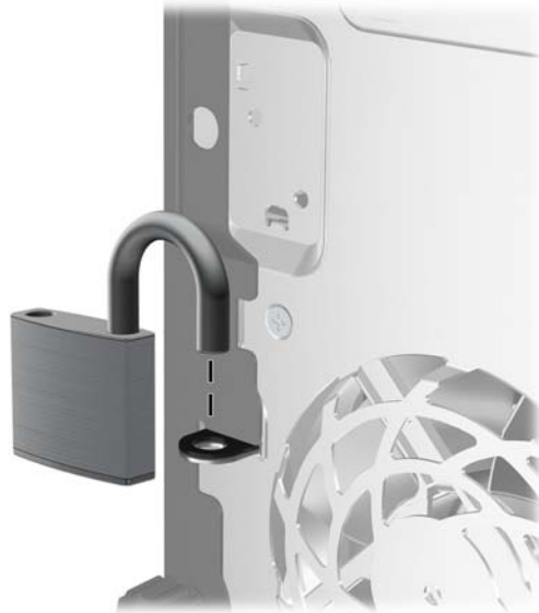
Figure 8-39 Installing a Padlock
