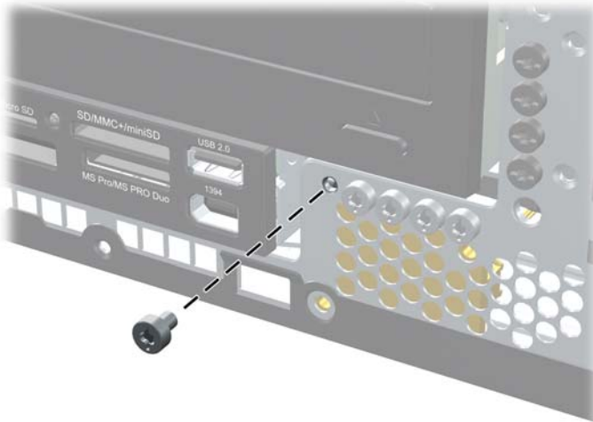
Figure 9-64 Retrieving the Front Bezel Security Screw
