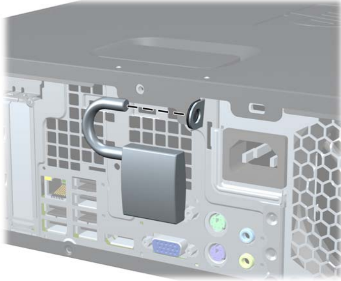
Figure 9-59 Installing a Padlock
