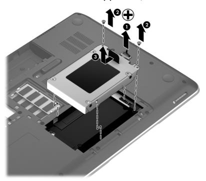
7. If it is necessary to replace the hard drive screws (1), hard drive bracket (2), or hard drive connector cable (3), remove and replace the components. The hard drive screws, hard drive bracket, and hard drive connector cable are available in the Hard Drive Hardware Kit, spare part number 682063-001.
