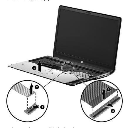
Reverse this procedure to install the keyboard.
