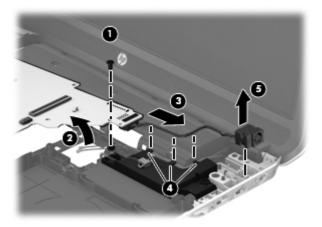
5. Remove the power connector cable.
