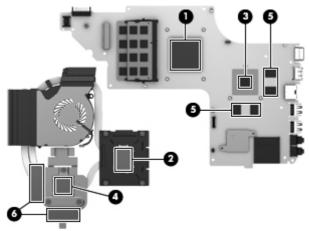
NOTE: The following illustration shows the replacement thermal material locations on a computer model equipped with an AMD processor and a graphics subsystem with UMA memory. Thermal paste is used on the processor (1) and the heat sink section (2) that services it.
