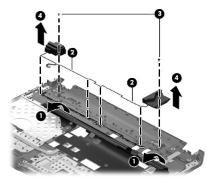
Reverse this procedure to install the top speakers.
