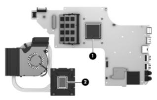
NOTE: The following illustration shows the replacement thermal material locations on a computer model equipped with an Intel processor and a graphics subsystem with discrete memory.
