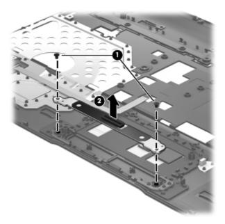
Reverse this procedure to install the TouchPad button board.
