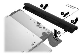
**8.** If it is necessary to replace the optical drive bracket, position the optical drive with the rear panel toward you.
