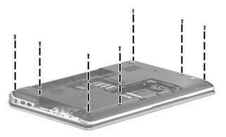
2. Remove the three Phillips PM2.5×5.5 screws that secure the top cover to the computer.
