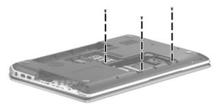
3. Remove the nine Phillips PM2.5×3.5 screws that secure the top cover to the computer.
