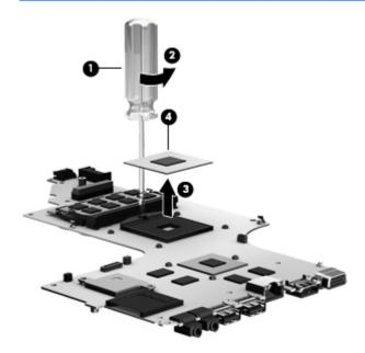
Reverse this procedure to install the processor.
