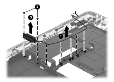
Reverse this procedure to install the optical drive connector cable.
