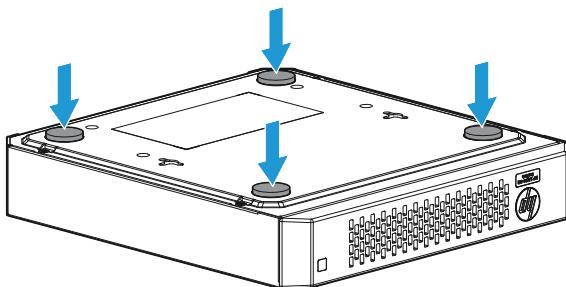
If you are mounting the switch on a wall or under a surface, do not attach the rubber feet.
