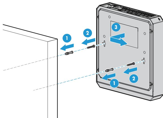
**Under-Surface Mounting:** Install the two screws on the surface bottom similarly to the procedures for wall mounting. Then, position the switch over the screws and slide to lock in place. Install the third screw at the side of the switch to prevent it from sliding out of the locked position, if necessary.
