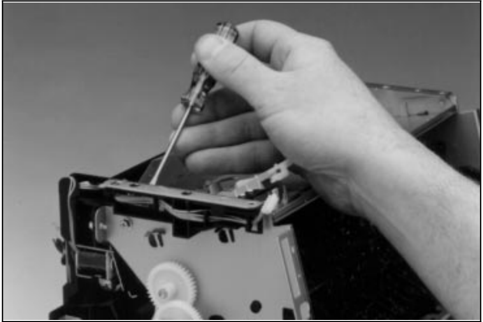
Paper Feed Frame Removal (2 of 4)
