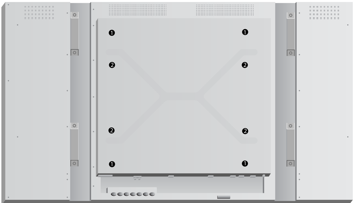
Figure 3-40 VESA mounting holes
