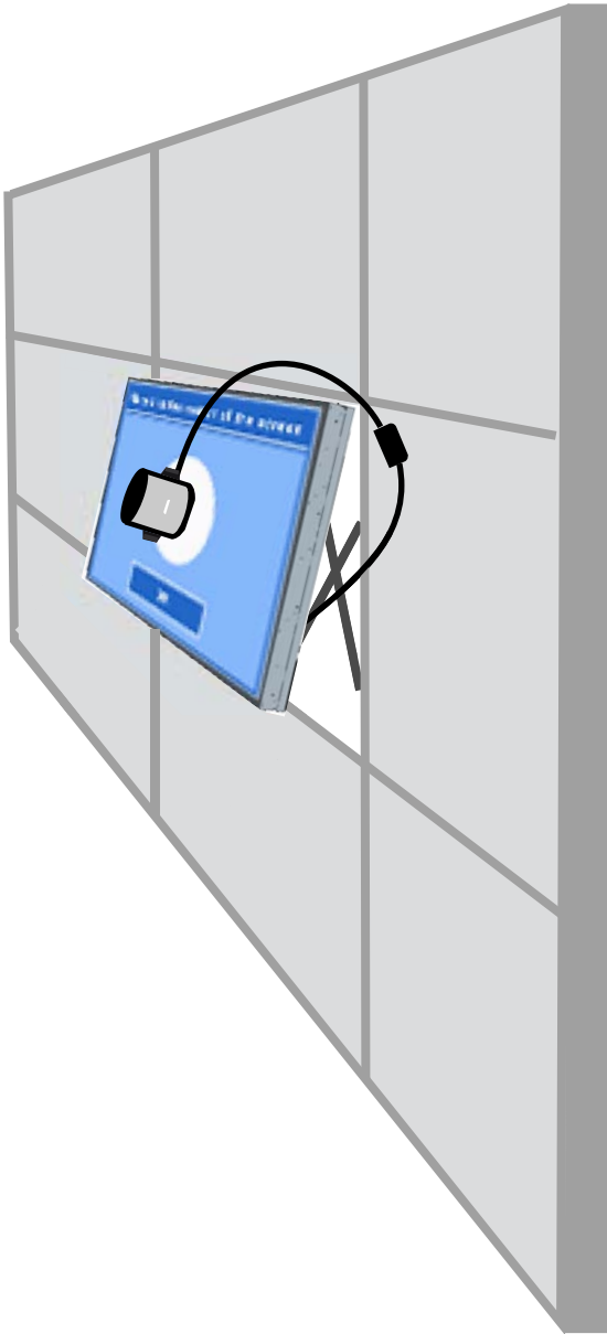
Figure 4-11 Positioning the colorimeter
