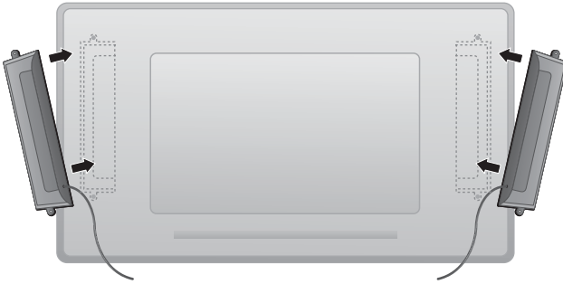
Figure 3-2 Mounting the speakers
