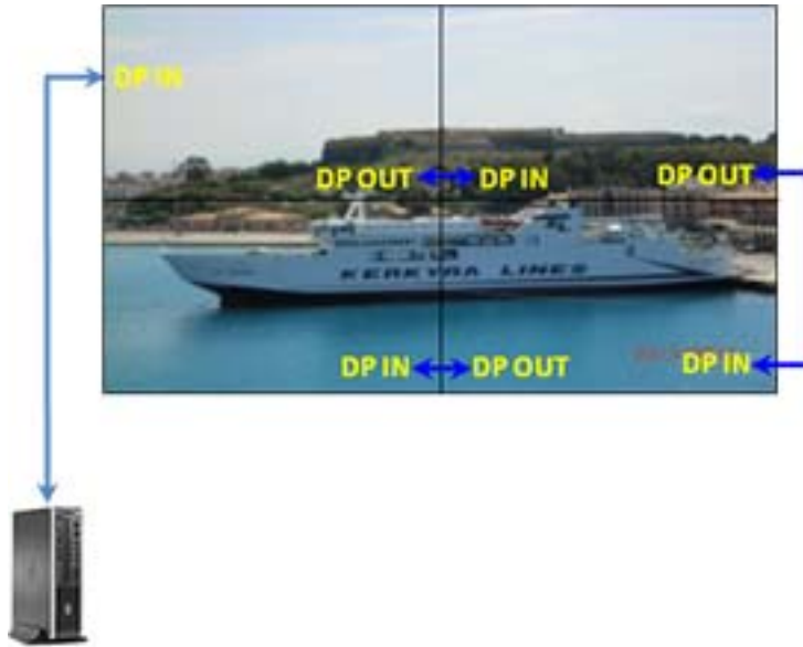
Figure 3-35 Daisy chain connection – DisplayPort
