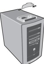
2 Remove the docking station cover by pressing the two tabs in the back of the cover and lifting up.
