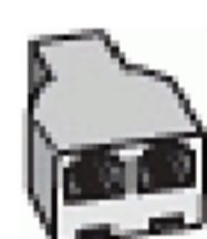
Figure B-16 Example of a parallel splitter
