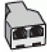
Figure B-17 Example of a parallel splitter
