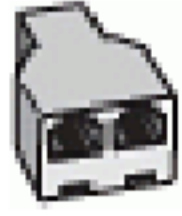
Figure B-11 Example of a parallel splitter
