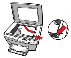
• If you are using an ADF, place your originals in the feeder with the printed side facing toward the back and with the top to the right. Align the paper with the right side of the ADF. Be sure to put full-sized pages only in the ADF, and adjust the page guide to the length of the originals.
