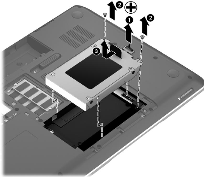
**NOTE:** After removing the hard drive from the computer, you must remove the hard drive bracket to access the hard drive itself.
