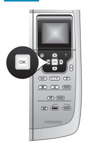
**a** Press **OK** at each of the prompts on the control panel to start print cartridge alignment.
