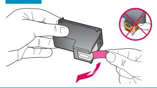
Pull the pink tab to remove the tape from **both** print cartridges.
