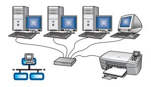
Use this connection type if you want an Ethernet cable connection between the device and your network.
