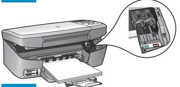
Lift the access door until it stops. The print carriage moves to the right.
