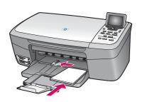
a Remove the plain white paper and load the 4 x 6 in (10x15 cm) photo paper. Place the paper glossy side down. Move the paper adjusters next to the stack of paper.
