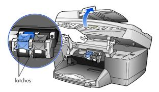
2 After the carriage stops moving, lift the latch to release the print cartridge, then pull it toward you out of its slot.
