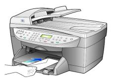
• If you are printing multiple envelopes, remove all paper from the main tray, and then slide a stack of envelopes into the tray, with the envelope flaps up and to the left (print-side down), until they stop.
