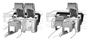
**6** Pull the end of the latch toward you, press down until it stops, and then release. Make sure the latch catches below the bottom tabs.
