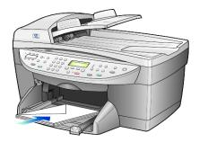
Adjust the paper-width guide against the envelopes (be careful not to bend the envelopes). Make sure the envelopes fit within the tray (do not overload it).
