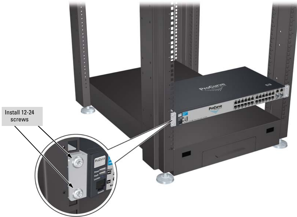
Figure 2-7. Mounting in a rack
