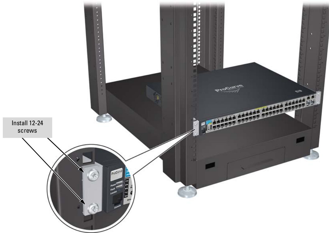
Figure 2-5. Mounting in a rack
