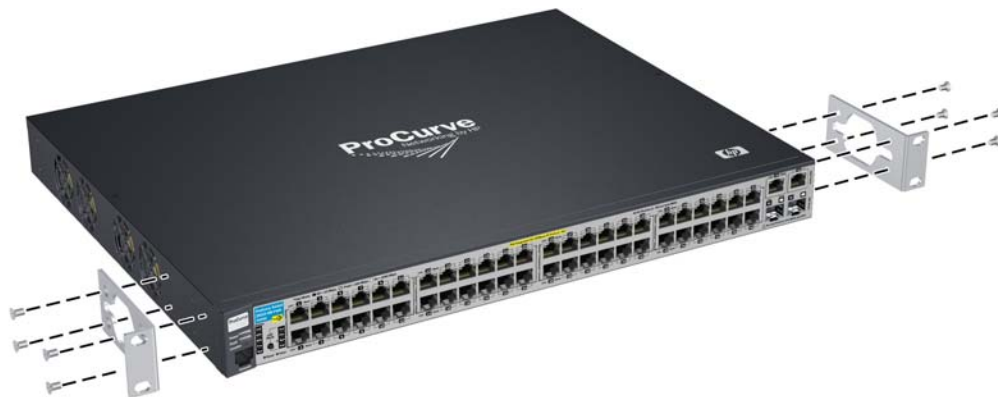
Figure 2-4. Attaching large mounting brackets
