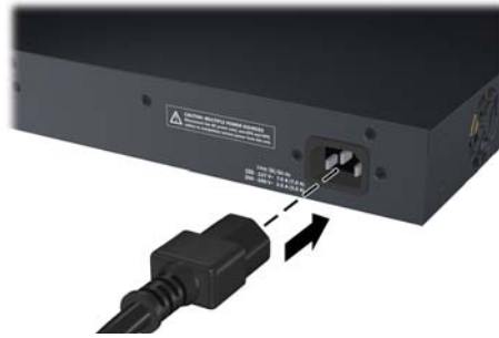
Figure 2-9. Connecting the power cord
