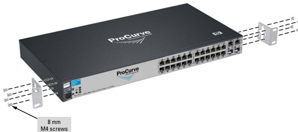
Figure 2-6. Attaching small mounting brackets
