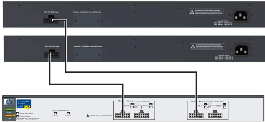
Figure 2-17. Connecting a 610 EPS to two 2610s EPS
