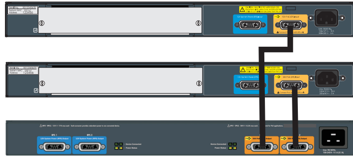
Figure 2-14. Connecting EPS to two 24-port switches.
