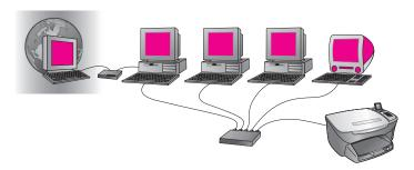
If you have this configuration, connect your HP PSC to the hub with an Ethernet cable and proceed to set up your hp psc for wired network use on page 134.
