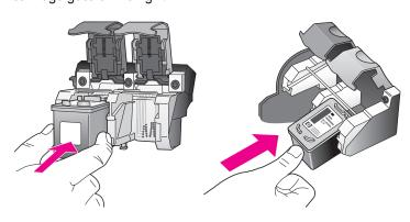
7 Press down on the latch until it stops. Make sure the latch catches below the bottom tabs.
