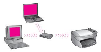
In this scenario, you can route the Internet connection directly through the access point using an Ethernet cable.
