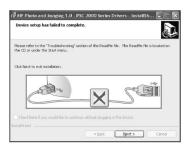
Normally, a green check appears indicating that the plug and play is successful. A red X indicates that the plug and play failed.
