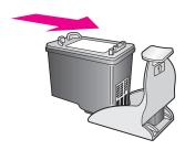
To remove the print cartridge from the print cartridge protector, press down and back on the top of the print cartridge protector to release the print cartridge, then slide the print cartridge out of the print cartridge protector.
