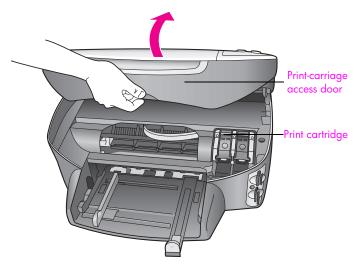
2 After the carriage stops moving and the ramp has lowered, lift the latch up to release the print cartridge.
