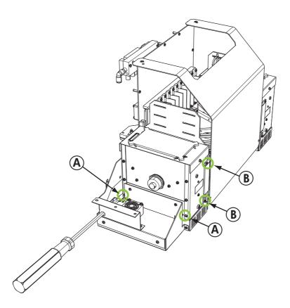
4. Lift up to remove the lamp housing from the printer.
