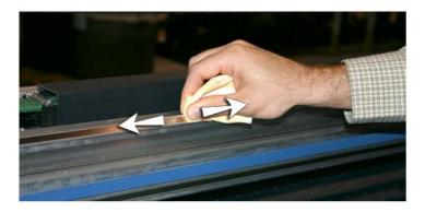
5. Lubricate behind the top area of the rail where the carriage wheels contact.
