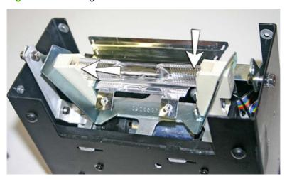
2. Tighten the two screws that hold the reflectors together (see <u>Figure 9-6 Reflector screws on page 63</u> for screw locations).
