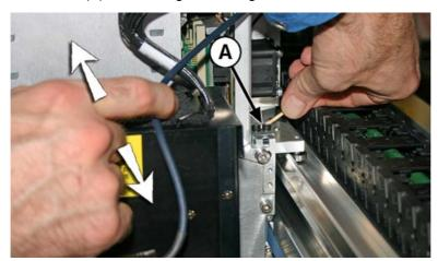
**6.** Clean the lower carriage wheel by placing an IPA moistened cotton swab next to the wheel and moving the carriage back and forth.
