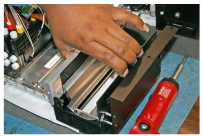
Once the lamp housing is installed into the lamp base, tighten the four screws that you loosened in the previous step.
