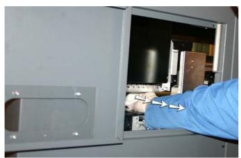
4. Fully saturate a lint-free cloth with printhead flush solution.
