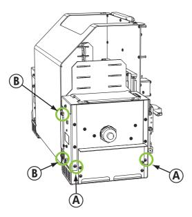
3. Lift up to remove the lamp housing from the printer.
