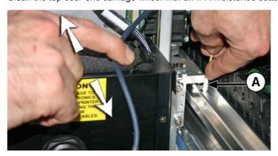
5. Clean the top slanted wheels by inserting an IPA moistened cotton swab into the opening above the wheels (A) and moving the carriage back and forth.
