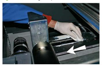
Using a lint-free cloth, clean both of the wiper rails on both sides of the wiper carriage.
