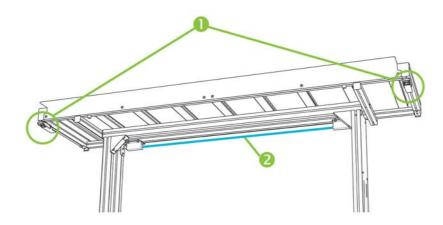
Optional extension tables are also available as an accessory, When properly assembled and attached to the ends of the standard tables, the extension tables enable safe and reliable handling of large media sheets. During use, the extension tables must be latched to the standard tables for
