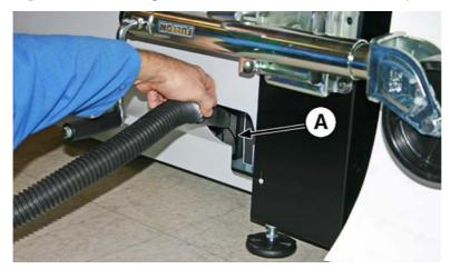
**4.** Vacuum the filter (A in photo below.) located under the printer's chassis near the power cord attachment point, and remove dust from the surrounding area.
