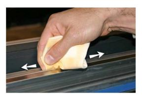
6. Using a lint-free cloth and Printhead Flush, clean the lower carriage-wheel strip from end to end on the rail (moving the carriage to clean the full length of the rail).
