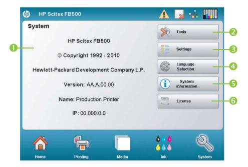
To switch to the System page, press the System icon in the Activity Tray at the bottom of the screen.
