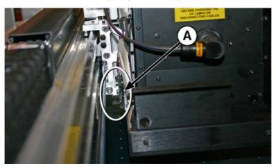
6. Locate the upper and lower slits of the optical sensor.
