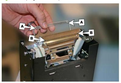
2. Loosen the two screws that hold the two reflectors together until the outside reflector can be removed.
