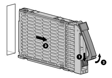
**CAUTION:** Populate hard drive bays with a SAS disk drive or a hard drive blank. Operating the server blade without a SAS disk drive or disk drive blank causes improper airflow and cooling, which can lead to thermal damage.
