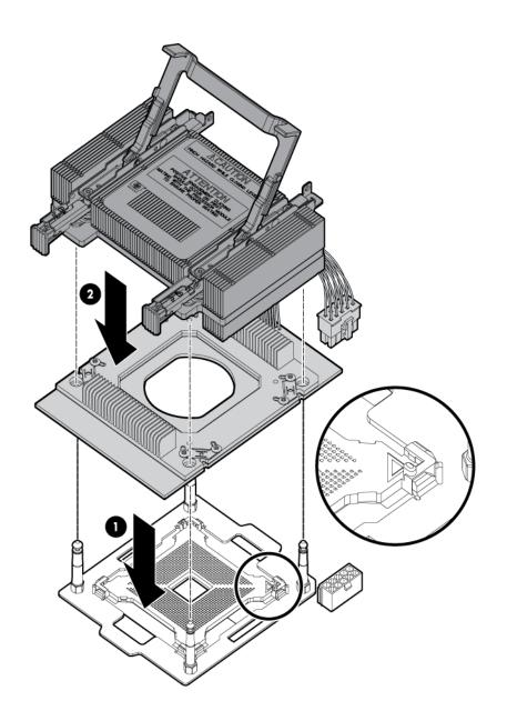
**CAUTION:** To prevent thermal instability and damage to the server blade, do not separate the processor module from the processor's heatsink after they have been coupled.
