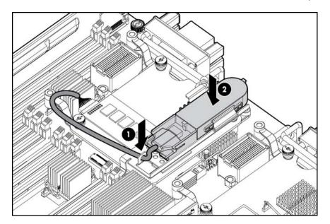
**NOTE:** After installing a BBWC battery, you might see a POST message during reboot indicating the array accelerator is temporarily disabled. This is normal as the new BBWC battery will have a low charge. The recharge process will begin automatically when the server blade is installed in the enclosure.
