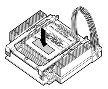
3. Install the processor over the load posts.
