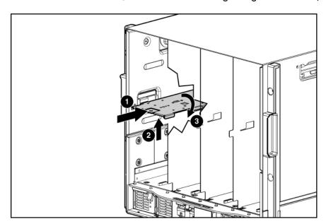
3. Lift the left side of the device bay shelf to disengage the three tabs from the divider wall, and then remove it from the enclosure.
