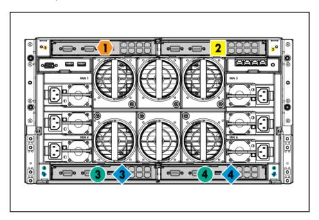
To support network connections for specific signals, install an interconnect module in the bay corresponding to the embedded NIC or mezzanine signals.
