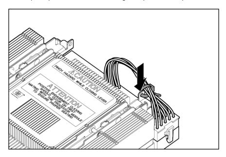
**CAUTION:** When the CPU is installed, dress all slack in the power cable to the connector end of the cable. Failure to do so could result in pinched or damaged CPU power cables.
