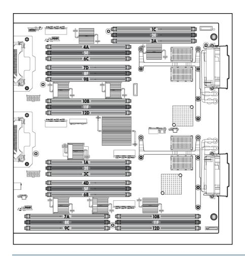
**NOTE:** The server blade ships with at least two DIMMs installed in slots 3A and 4A.
