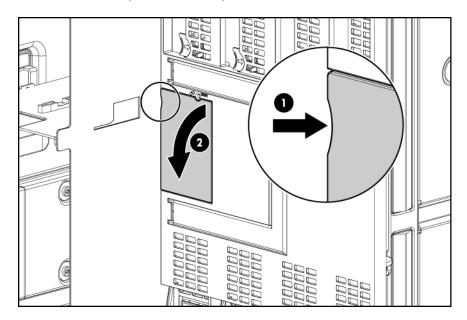
For more information see "Installing the Blade Link for BL870c i2 or BL890c i2 configurations" (page 22)
