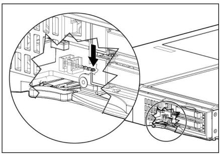
**NOTE:** The iLO heartbeat LED is visible when looking through the front grill of the Blade Link nearest to the hard drive bays.
