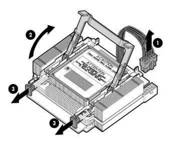
6. Lift the CPU and heatsink off of the socket, pulling straight up.
