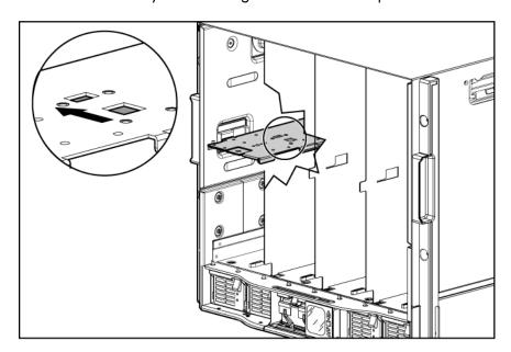
2. Push the device bay shelf back until it stops, lift the right side slightly to disengage the two tabs from the divider wall, and then rotate the right edge downward (clockwise).
