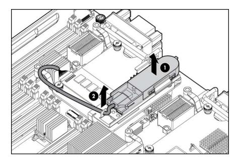
8. Push the battery plug out of the battery connector.
