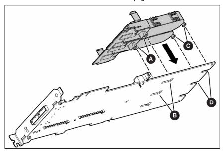
Slide the batteries toward the board bracket until the connectors on the cache module are firmly seated in the DIMM connector. (When the cache module is correctly seated, the gold contacts on the cache module are completely hidden within the DIMM connector.)
