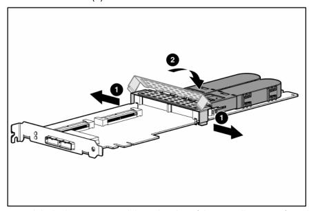
Slide the batteries toward the right edge of the controller, away from the bracket.
