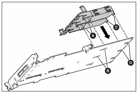
Slide the batteries toward the board bracket until they are firmly seated against the connectors on the cache module.
