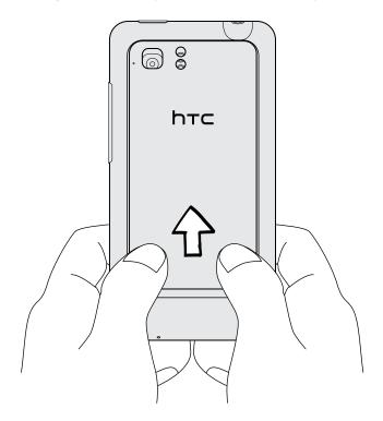
3. With your finger, lift up the back cover from the bottom side to remove it.
