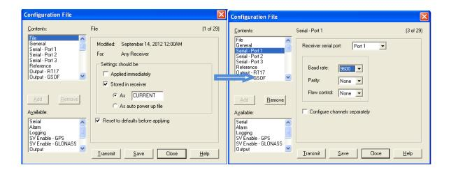
Click on 'Output' under the Available selection box → Click Add to enable Output type selection→ Select NMEA, Port 1 and appropriate Baud Rate
