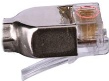
Figure 5-34 Unparallel contact strips of different heights
