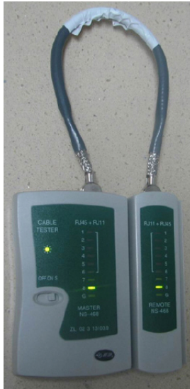
Figure 5-39 Testing the conduction and connections of wires
