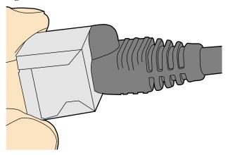
**Step 4** To remove an Ethernet connector, press the locking key and pull out the connector, as shown in **Figure 5-126**.
