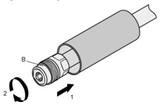
**Step 5** Mount the body of the connector onto the feeder cable so that the inner conductors of the connector and feeder cable are connected. Use a spanner (27 N•m to 30 N•m torque recommended) to fasten the body and back shell, as shown in **Figure 5-93**.
