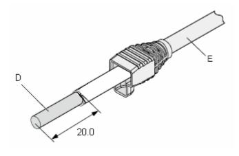
**Step 3** Pull outward the shielded aluminum foil and cut off the PET membrane and ground cables along the end face of the outer jacket, as shown in **Figure 5-68**.
