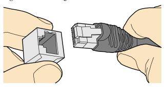
Step 2 Insert the male connector into the female connector, as shown in Figure 5-124.
