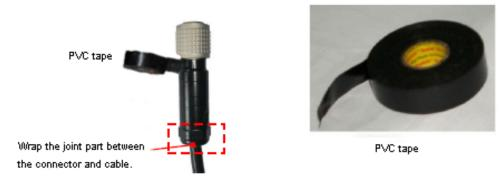
2. Wrap three layers of insulation tape, as shown in Figure 5-118.
