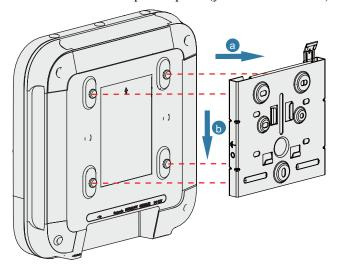
In a scenario with heavy vibrations, tighten the AP to the mounting bracket using M4x30 screws with a torque of 1.4N•m. This prevents the AP falling off from due to vibrations. In normal scenarios, you do not need to install these screws.
