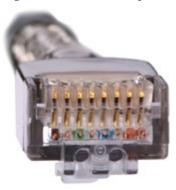
**Step 2** Hold an RJ45 connector and turn it 45°. Observe the top edges of the metal contact strips. **Figure 5-81** shows an unqualified piece.
