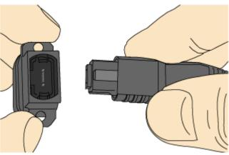
Step 3 Hold the shell labeled "PUSH" and feed the male connector into the female connector until you hear a clicking sound. The male and female connectors are securely installed, as shown in Figure 5-143.
