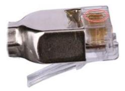
**Step 3** Check whether the contact strips are clean. If they are not clean and the dirt cannot be removed, replace it with a new RJ45 connector. **Figure 5-82** shows an unqualified piece.
