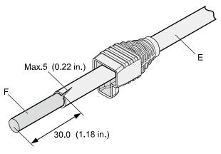
**Step 3** Fit the metal shell onto the twisted-pair cable. The shield layer is covered by the metal shell, as shown in **Figure 5-39**.
