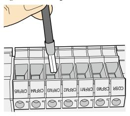
**Step 2** Insert the terminal into the jack vertically, and turn the screw clockwise to fasten the terminal, as shown in **Figure 5-115**.
