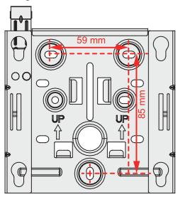
2. Use a 6 mm drill bit to drill 25 mm to 30 mm deep holes in the drilling positions. Hammer the expansion tubes into the holes until the expansion tubes are completely embedded into the wall.
