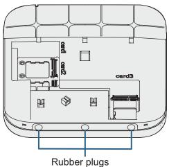
3. Place IoT cards in the slots and tighten the cards using M2x7 screws (with a tightening torque of 1.5 N•m). You are advised to start installation from the card1 slot.
