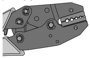
**Step 6** Hold the handles of the COAX crimping tools with one hand. Tighten the two fastening screws clockwise. **Figure 5-150** and **Figure 5-151**shows the mold installed in the COAX crimping tool.
