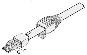
Figure 5-44 Connections between wires and pins
