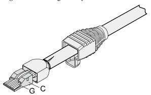
**Step 8** Put the connector body onto the wire holder and turn the metal shell by 90°, as shown in **Figure 5-46**.
