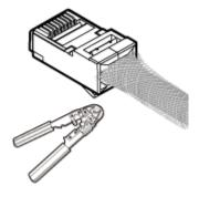
Figure 5-56 Neatly cutting braid shields
