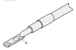
**Step 5** Push the heat shrink tubing toward the connector until the tube covers the crimped part, and then use a heat gun to heat the tube, as shown in **Figure 5-31**.
