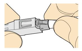
**Step 5** To disassemble an LC fiber connector, press the locking nut to release the locking clips from the bore, and gently pull the male connector, as shown in **Figure 5-138**.
