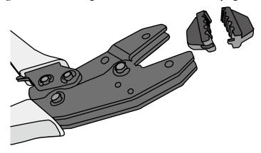
**Step 4** Place the mold to be installed into the jaw of the COAX crimping tools and align the screw holes, as shown in **Figure 5-148**.
