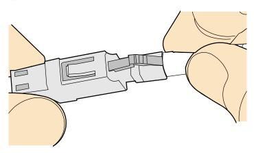
**Step 4** A clicking sound indicates that the male connector is locked, as shown in **Figure 5-137**.
