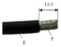
Step 2 Route the Cable jacket (E) through the nut (D), as shown in Figure 5-98.
