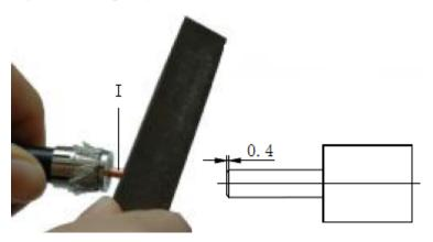
Step 8 Use a brush to remove impurities from the cross section of the feeder, as shown in **Figure** 5-104.
