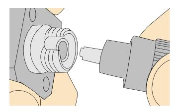
**Step 3** Align the male connector with the female connector and gently push the male connector until it is completely seated in the female connector, as shown in **Figure 5-132**.
