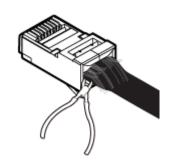
**Step 7** Repeat **Step 1** through **Step 6** to assemble the optimized shielded RJ45 connector on the other end of the network cable.
