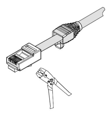
**Step 7** Move the connector jacket to the connector body to wrap the connector shell, as shown in **Figure 5-74**.
