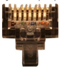
**Step 5** Hold the connector with the side facing towards you, and check whether you can see the cross-sections of the wires. Ensure that the ends of the wires are in good contact with the edge of the RJ45, and that the contact strip blade extends beyond the ends of the wires and is crimped with the wires. If not, replace the connector. **Figure 5-84** shows an unqualified piece.
