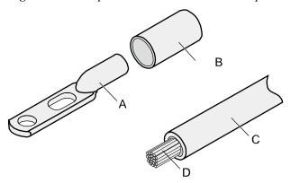
A. JG terminal B. Heat-shrinkable tubing C. Insulation layer of a power cable
