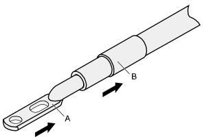
**Step 3** Put the bare crimping terminal onto the exposed conductor, and ensure that the bare crimping terminal is in good contact with the insulation of the power cable, as shown in **Figure 5-29**.
