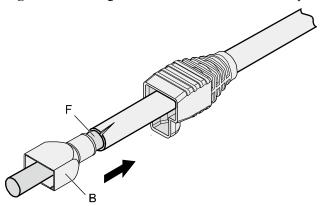
**Step 4** Fit the metal shell onto the twisted-pair cable until the shield layer is covered completely. Along the edge of the metal shell, cut off the aluminum foil shield layer and ensure that there is no surplus copper wire. The exposed twisted-pair cable is about 20 mm (0.79 in.) long, as shown in **Figure 5-40**.
