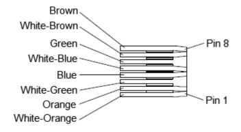
Figure 5-70 Neatly cutting the twisted pair
