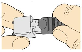
**Step 3** When you hear a click, the cable connector is completely inserted in the port. (The clip on the cable connector pops up to fix the connector in the port.) Pull the connector slightly and ensure that it is securely connected, as shown in **Figure 5-125**.
