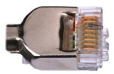
**Step 4** Check whether the contact strips and the plastic separators are well aligned and intact. If a separator is skewed and cannot be fixed, replace it with a new RJ45 connector. **Figure 5-83** shows an unqualified piece.
