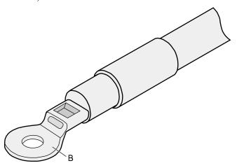
**Step 5** Push the heat shrink tubing (A) toward the connector until the tube covers the crimped part, and then use a heat gun to heat the tube, as shown in **Figure 5-26**.
