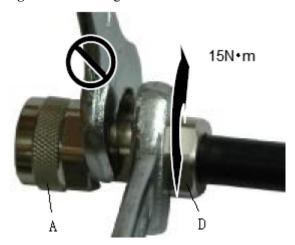
**Step 11** Figure 5-107 shows the effect drawing after the assembling is complete.
