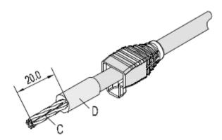
**Step 4** Arrange the twisted core wires according to color order shown in **Figure 5-69**. Use cutting pliers to neatly cut the front end of the twisted pair, as shown in **Figure 5-70**. **Figure 5-71** shows pin arrangement of each contact of the connector.
