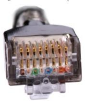
Figure 5-80 Contact strips of the same height
