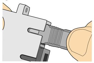
**Step 4** To disassemble an SC fiber connector, hold the shell of the connector (do not hold the fiber) and gently pull the connector in the direction vertical to the adapter. Unlock the male connector, and then separate it from the shell, as shown in **Figure 5-141**.
