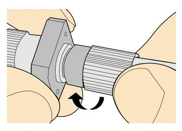
**Step 5** To disassemble an FC fiber connector, loosen the locking nut counterclockwise, and gently pull the male connector, as shown in **Figure 5-134**.
