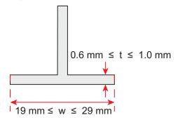
1. Remove two ceiling tiles around the T-rail, use screws to fix the adjustable buckle to the mounting bracket, hook the adjustable buckle to the T-rail, and secure the screw on the adjustable buckle to fasten the mounting bracket and T-rail.
