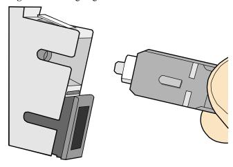
**Step 3** Feed the fiber connector into the female connector, with your fingers holding the shell of the fiber connector (not the pigtail). When you hear a click, the fiber connector is secured by the clips (internal parts, not illustrated in the figure). Pull the fiber connector gently. If the connector does not loosen, the installation is complete. See **Figure 5-140**.
