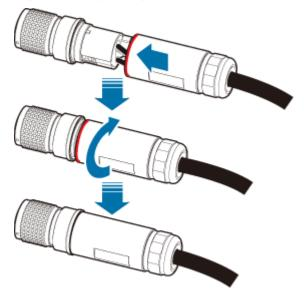
**Step 8** Pre-tighten the nut and socket and further tighten the nut using a torque wrench (opening width: 28 mm), as shown in **Figure 5-19**.
