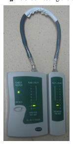
Step 3 Gently shake the connector and repeat Step 2 to check whether the metal contact strips are in good contact with the core wires and Ethernet ports, as shown in Figure 5-87.
