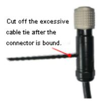
**Step 2** Fix the DC power cable connector to the PWR port, as shown in **Figure 5-122**. Ensure that positive and negative polarities are correct during the installation.
