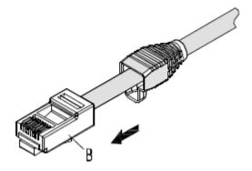
**Step 6** Use the crimping tool dedicated for FTP network cables to crimp the connector and neatly cut the aluminum foil along the end face of the connector, as shown in **Figure 5-73**.
