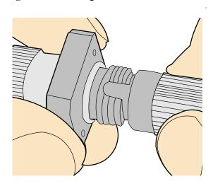
**Step 4** Fasten the locking nut clockwise and ensure that the connector is securely installed, as shown in **Figure 5-133**.
