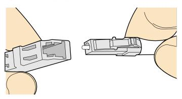
**Step 3** Align the male connector with the fiber adapter and gently push the male connector until it is completely seated in the fiber connector, as shown in **Figure 5-136**.
