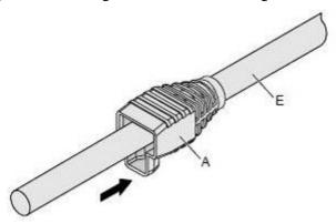
**Step 2** Strip 20 mm outer jacket off the cable and cut off the nylon layer inside the jacket, as shown in **Figure 5-67**.
