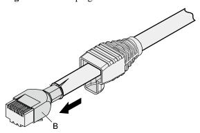
**Step 10** Push the jacket towards the metal shell until the metal shell is covered. This completes the assembly of one end of the cable, as shown in **Figure 5-48**.
