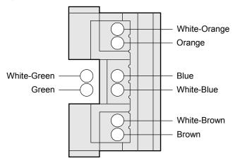
**Step 6** Align the four pairs of cables in the holder, as shown in **Figure 5-43**. The connections between the wires and the pins are shown in **Figure 5-44** and listed in **Table 5-6**.
