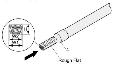
**Step 4** Check the maximum width of the tubular crimped terminal. The maximum width of a tubular crimped terminal is listed in **Table 5-5**.
