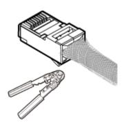
Step 5 Neatly cut braid shields exposed out of the connector along the load bar, as shown in **Figure** 5-62.
