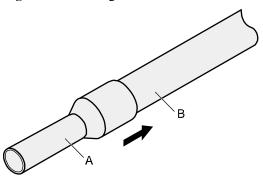
Step 3 Crimp the joint parts of the cord end terminal and the conductor, as shown in Figure 5-35.
