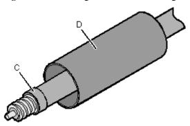
**Step 4** Put the back shell of the connector onto the feeder cable. Tighten the back shell to the end of the feeder cable, as shown in **Figure 5-92**.
