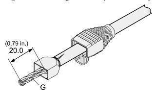
Step 5 Lead the four pairs of twisted-pair wires through the wire holder, as shown in Figure 5-41 and Figure 5-42. Ensure that the colored wires are in the correct location in the cable.
