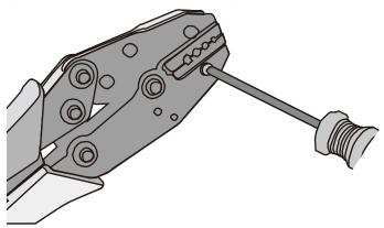
**Step 2** Hold the handles of the COAX crimping tools to open the self-locking mechanism. The jaw of the COAX crimping tools opens automatically, as shown in **Figure 5-146**.
