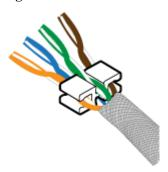
Step 3 Hold the arranged core wires and route them through the load bar, as shown in Figure 5-52.
