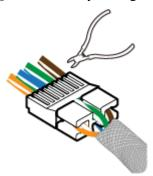
Step 5 Insert the load bar into the RJ45 connector, as shown in Figure 5-54.
