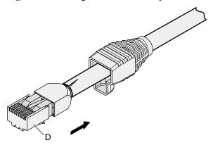
**Step 9** Push the metal shell toward the connector body until the wire holder and the connector body are engaged completely. Crimp the connector, as shown in **Figure 5-47**.
