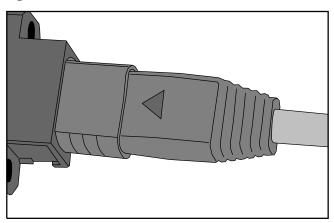
**Step 4** To disassemble an MPO fiber connector, hold the shell labeled "PULL" and remove the male connector, as shown in **Figure 5-144**.
