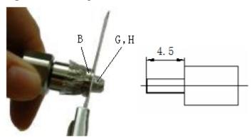
Step 7 Use the file to taper the internal conductor (I) of the feeder, as shown in Figure 5-103.
