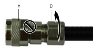
**Step 10** Use a wrench to fix the nut (D) to connector's main body (A) with recommended tightening torque 15 N•m, as shown in **Figure 5-106**.
