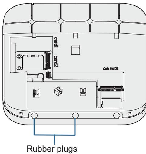
3. Place the card in the card1 slot and tighten the card using M2x7 screws (with a tightening torque of 1.5 N•m).
