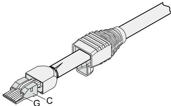
**Step 8** Put the connector body onto the wire holder and turn the metal shell by 90°, as shown in [Figure 5-46](#).
