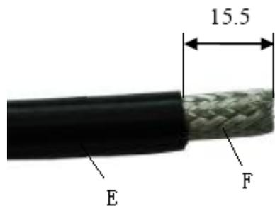
**Step 2** Route the Cable jacket (E) through the nut (D), as shown in [Figure 5-98](#).
