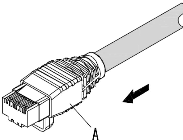
**Step 8** Repeat **Step 1** through **Step 7** to assemble the shielded RJ45 connector on the other end of the network cable.
