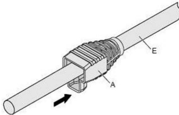
**Step 2** Strip 20 mm outer jacket off the cable and cut off the nylon layer inside the jacket, as shown in [Figure 5-67](#).
