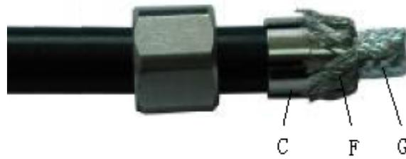
**Step 5** Install the lining (B) on the feeder and tightly crimp the shielded layer (F) of the feeder, as shown in [Figure 5-101](#).
