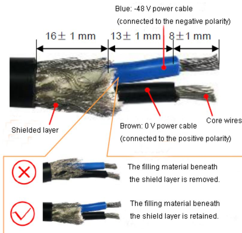
**Step 3** Open the clip and correctly insert the core wires to the negative and positive holes, as shown in [Figure 5-4](#).
