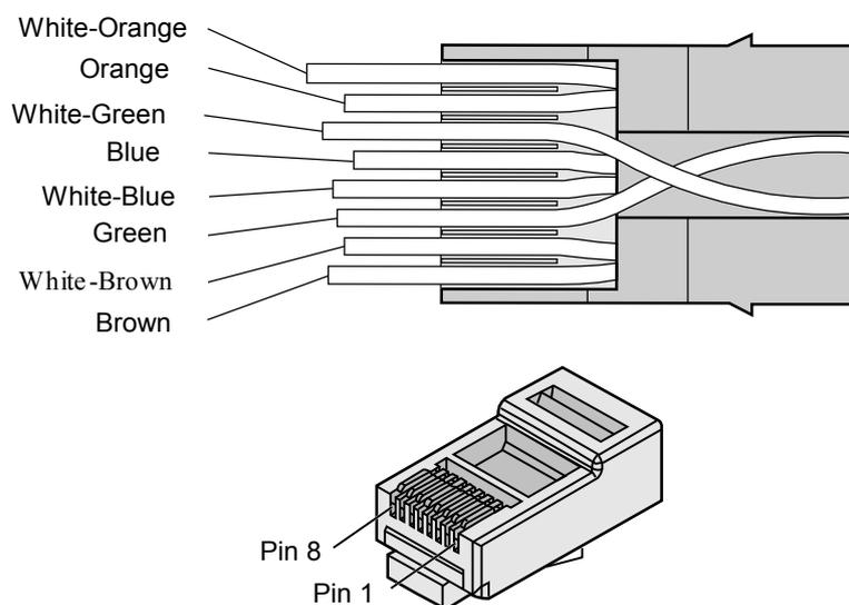
**Table 5-6** Connections between wires and pins (using a straight-through cable as an example)
