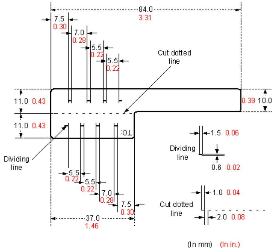
To specify more clearly the position of a cable, use the dividing lines on the label. For example, there is a dividing line between the cabinet number and the chassis number, and another one between the chassis number and the slot number. Each dividing line is light blue (Pantone 656c) and 1.5 mm x 0.6 mm (0.06 in. x 0.02 in.).
