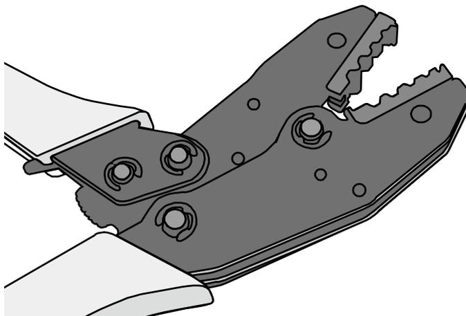
**Step 3** Remove the mold from the COAX crimping tools, as shown in [Figure 5-147](#).
