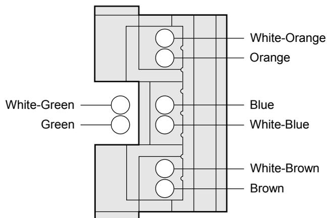
**Step 6** Align the four pairs of cables in the holder, as shown in [Figure 5-43](#). The connections between the wires and the pins are shown in [Figure 5-44](#) and listed in [Table 5-6](#).
