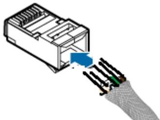
**Step 4** Use the crimping tool to crimp the connector, as shown in [Figure 5-61](#).
