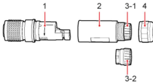
1. Enclosure      2. Socket      3-1. Clamping jaw 1      3-2. Clamping jaw 2      4. Nut
