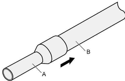
**Step 3** Crimp the joint parts of the cord end terminal and the conductor, as shown in **Figure 5-35**.
