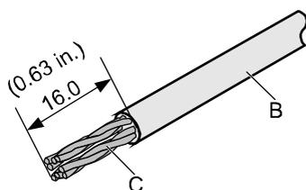
**Step 2** Align the four pairs of wires and cut the ends neatly, as shown in [Figure 5-77](#). The connections between the wires and the pins are listed in [Table 5-9](#).
