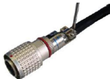
**Step 6** Pre-tighten the socket and enclosure and use the Phillips screwdriver to tighten the socket with the tightening torque no less than 1.2 N•m, as shown in [Figure 5-7](#).
