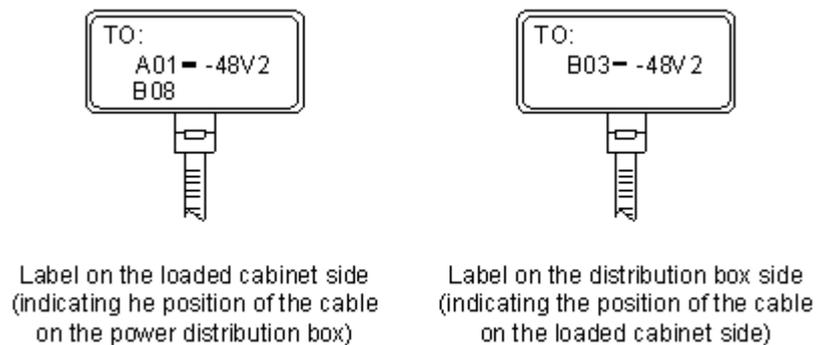
The meaning of the label in **Figure 5-166** is as follows:
