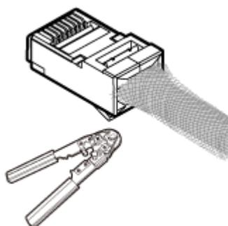
**Figure 5-56** Neatly cutting braid shields
