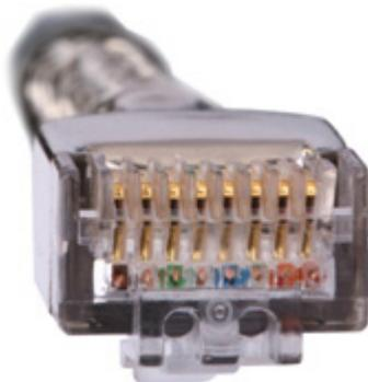
**Step 2** Hold an RJ45 connector and turn it 45°. Observe the top edges of the metal contact strips. **Figure 5-81** shows an unqualified piece.
