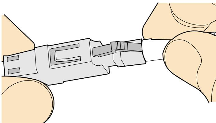
**Step 4** A clicking sound indicates that the male connector is locked, as shown in [Figure 5-137](#).
