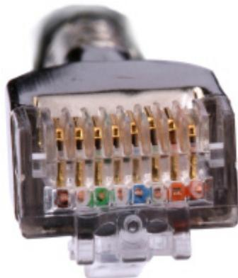
**Figure 5-80** Contact strips of the same height
