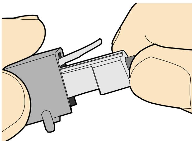
**Step 3** A crisp click indicates that the connector is locked by the locking key. Pull the connector slightly and ensure that it is securely connected. [Figure 5-129](#) shows an installed Ethernet connector.
