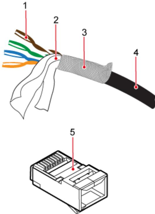
1: Core wires    2: Aluminum foil    3: Braid shield    4: Outer jacket    5: RJ45 connector
