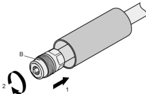
**Step 5** Mount the body of the connector onto the feeder cable so that the inner conductors of the connector and feeder cable are connected. Use a spanner (27 N•m to 30 N•m torque recommended) to fasten the body and back shell, as shown in [Figure 5-93](#).
