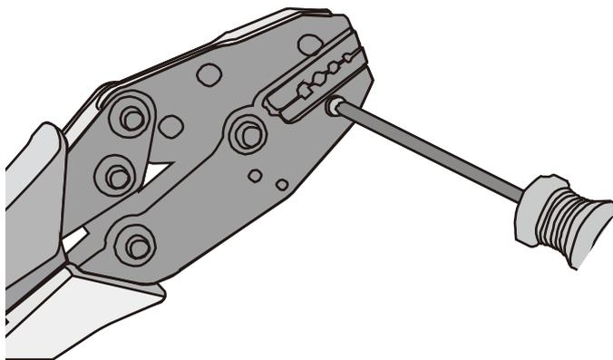
**Figure 5-151** An installed mold
