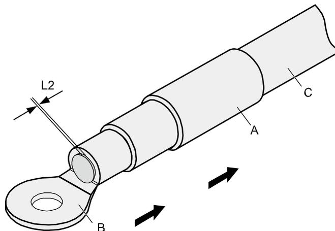
**Step 3** Put the OT terminal B onto the exposed conductor, and ensure that the OT terminal is in good contact with the insulation coating C, as shown in [Figure 5-24](#).
