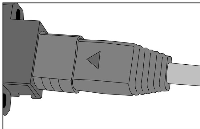
**Step 4** To disassemble an MPO fiber connector, hold the shell labeled "PULL" and remove the male connector, as shown in [Figure 5-144](#).
