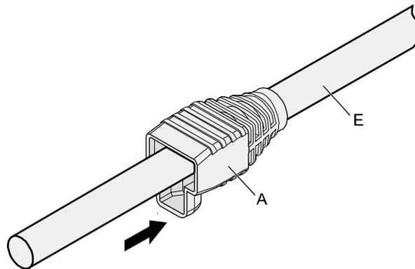
**Step 2** Remove a 30 mm (1.18 in.) long section of the jacket, cut off the nylon twine inside the jacket, and cut a no more than 5 mm (0.20 in.) cleft in the jacket, as shown in [Figure 5-38](#).
