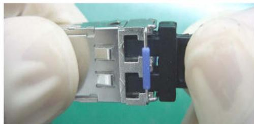
If no protective cap is available, use fibers to protect the optical module, as shown in [Figure 5-171](#).
