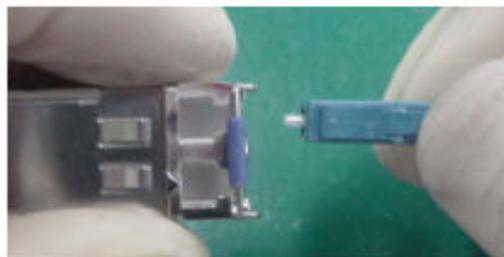
3. Cover unused optical connectors with protective caps, as shown in [Figure 5-172](#), and then lay out fibers on the fiber rack or coil them in a fiber management tray to prevent fibers from being squeezed.
