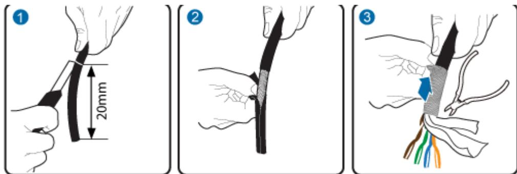
**Step 2** Arrange the twisted pair wires in the order of colors shown in [Table 5-8](#) and cut the wire ends neatly with 12 mm core wires left, as shown in [Figure 5-59](#).
