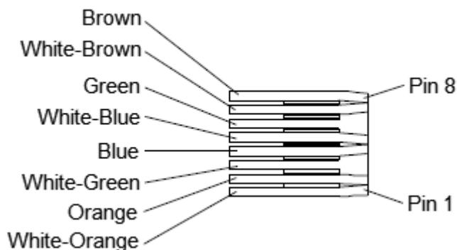
**Figure 5-70** Neatly cutting the twisted pair
