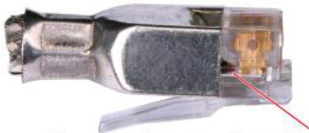
Not in good contact with the edge of the RJ45 trough
