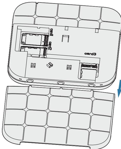
2. Remove rubber plugs based on the number of IoT cards to be installed. One rubber plug maps one IoT card.
