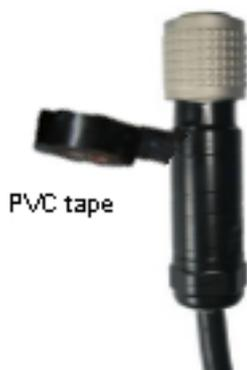
4. Tightly bind the PVC tape at the ends of the wrapping section, as shown in [Figure 5-121](#).
