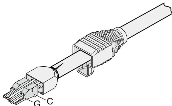
**Figure 5-44** Connections between wires and pins
