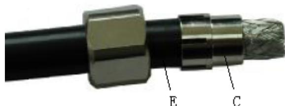
**Step 4** Peel off the shielded layer (F) to the direction of the clip (C) so that the aluminum foil (G) is exposed, as shown in [Figure 5-100](#).
