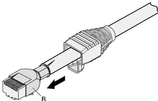
**Step 10** Push the jacket towards the metal shell until the metal shell is covered. This completes the assembly of one end of the cable, as shown in [Figure 5-48](#).
