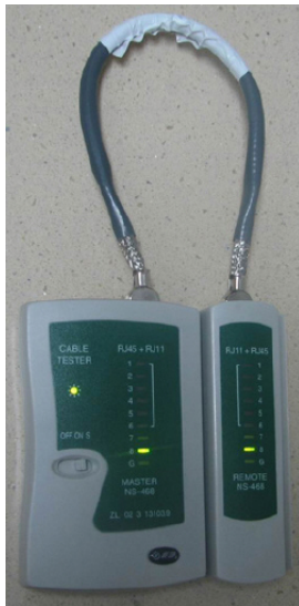
Figure 5-39 Testing the conduction and connections of wires
