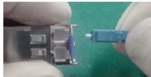
Figure 5-98 Using fibers to protect an optical module
