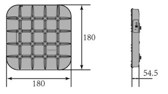
Figure 2-1 Dimension of AP4130DN (Unit: mm)
