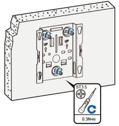
3. Align the mounting screws at the rear of the AP with the mounting holes on the mounting bracket and hang the AP on the bracket. Press the AP downwards to secure the AP on the wall.
