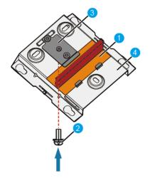
2. Hang the AP on the mounting holes by aligning the mounting screws at the rear of the AP with the mounting screws on the bracket and push the AP horizontally to secure the AP.
