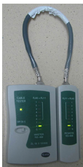
Figure 5-39 Testing the conduction and connections of wires
