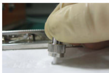
Figure 5-96 Cleaning optical fibers with special cleaning tissues
