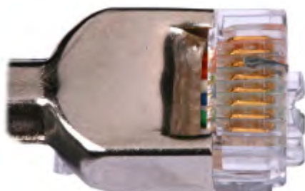
Figure 5-35 Dirt on a contract strip
