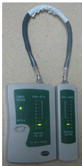
Figure 5-39 Testing the conduction and connections of wires
