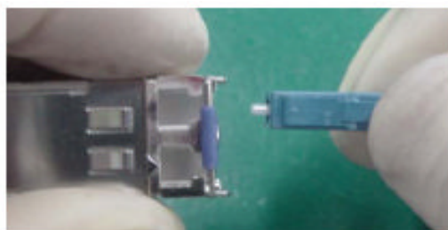
Figure 5-98 Using fibers to protect an optical module
