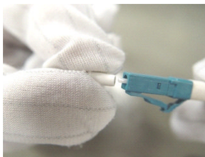
Figure 5-99 Installing a protective cap on a fiber
