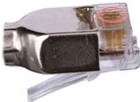
Figure 5-34 Unparallel contact strips of different heights
