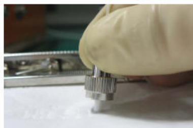
Figure 5-96 Cleaning optical fibers with special cleaning tissues
