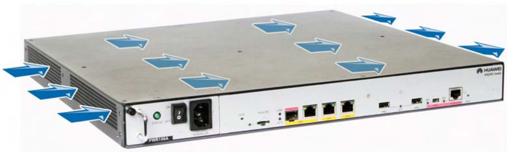
Figure 4-2 Air circulation through the AR2220-S chassis
