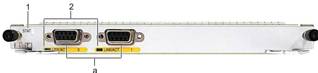
Figure 5-11 Appearance of the 2E1T1-M (WSIC)
