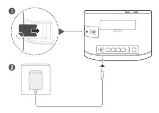
Insert a SIM card into the SIM card slot as shown in the preceding diagram and then connect the power adapter to the B<sub>315</sub> router. The router will turn on automatically and search for available mobile networks.
