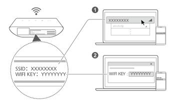
Once the router has connected to a mobile data network, you can connect your computer or mobile phone to the router's Wi-Fi network to access the Internet. Please refer to the label on the bottom of the router for the default wireless network name (SSID) and password (WIFI KEY).
