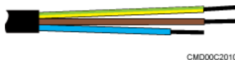
Figure 14-13 Stripping the jacket off the core wires of the power cable for the SPM60A
