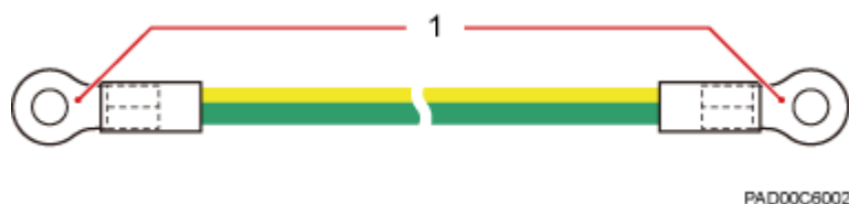
Figure 4-1 PGND cable appearance
