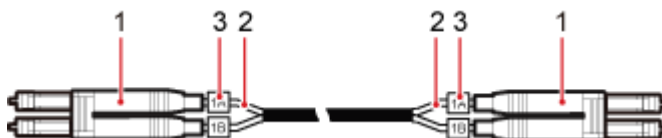
Figure 4-6 FE/GE fiber optic cable (2)
