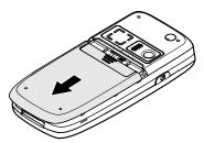
2. Press the battery release latch down and take out the battery.
