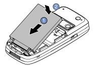
3. Press the battery down into the compartment and then slide back the cover.
