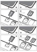
Do not insert or remove the SIM card when your device is powered on.
