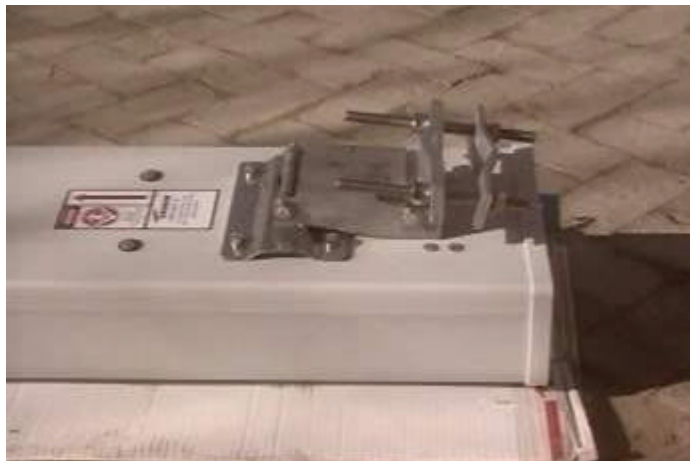
Figure 6-12 Fixing clip for the directional antenna
