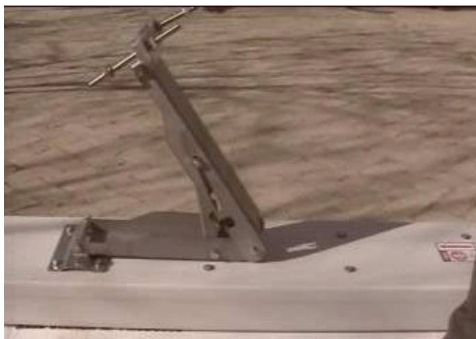
Figure 6-13 Adjusting device for the pitch angle of directional antenna
