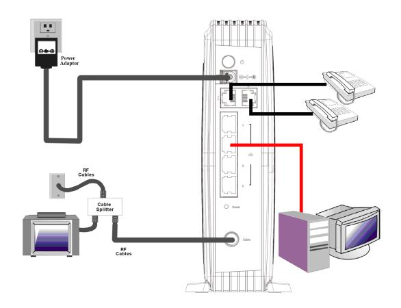
Fig. How to set up your connection
