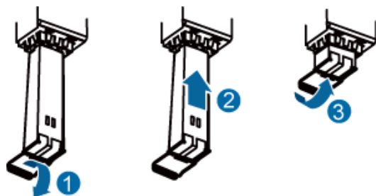
Figure 7-15 Installing an optical module
