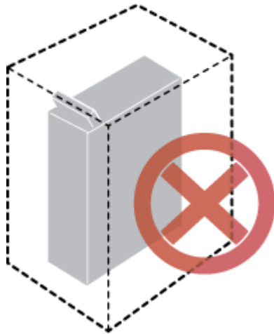
Figure 3-4 Improperly installed DRHs
