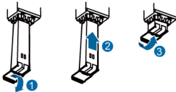
Figure 8-15 Installing an optical module
