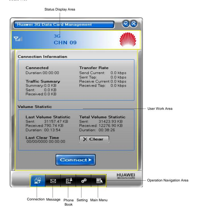
The interface is divided into three parts. From the top to down, they are Status Display Area, User Work Area, and Operation Navigation Area.
