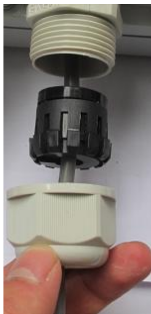
Figure 3-18 Installing the PG-head screw cap and air-proof block
