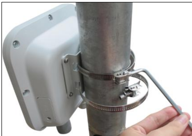
Figure 3-5 Adjusting the length of the hose clamp
