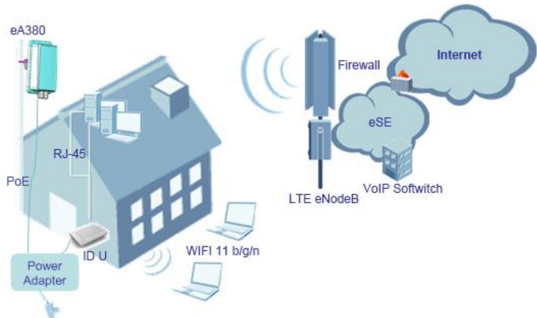
Figure 1-1 The eA380 deployed in wISP network
