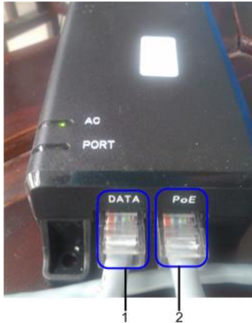
Figure 3-16 Connecting the PoE adapter
