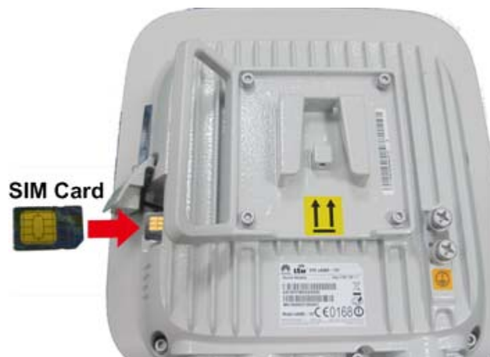
Figure 3-11 Installing the SIM card
