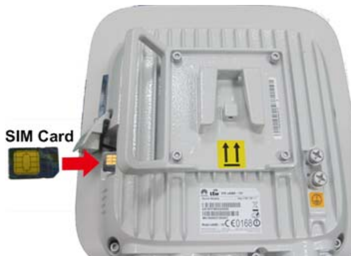
Figure 3-3 Installing the SIM card
