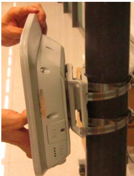
Figure 3-7 Installing the eA660 on the wall-mounting frame
