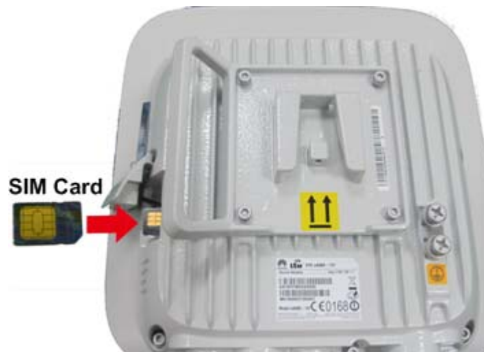
Figure 3-23 Installing the SIM card
