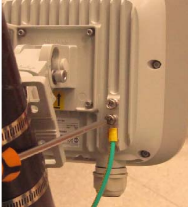
Figure 3-38 Connecting the ground cable
