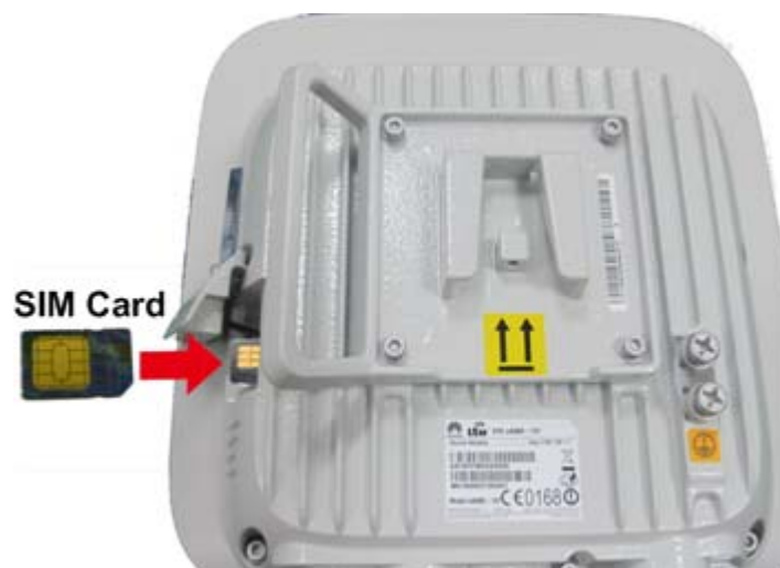
Figure 3-32 Installing the SIM card
