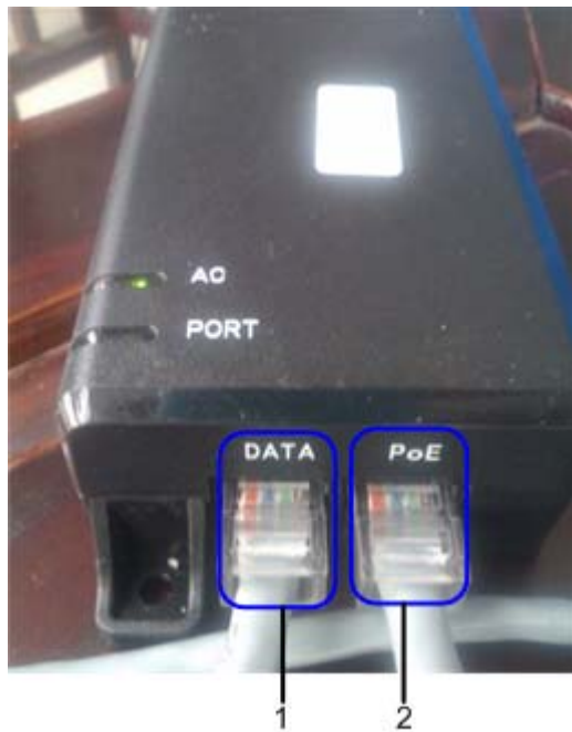
Figure 3-42 Connecting the PoE adapter
