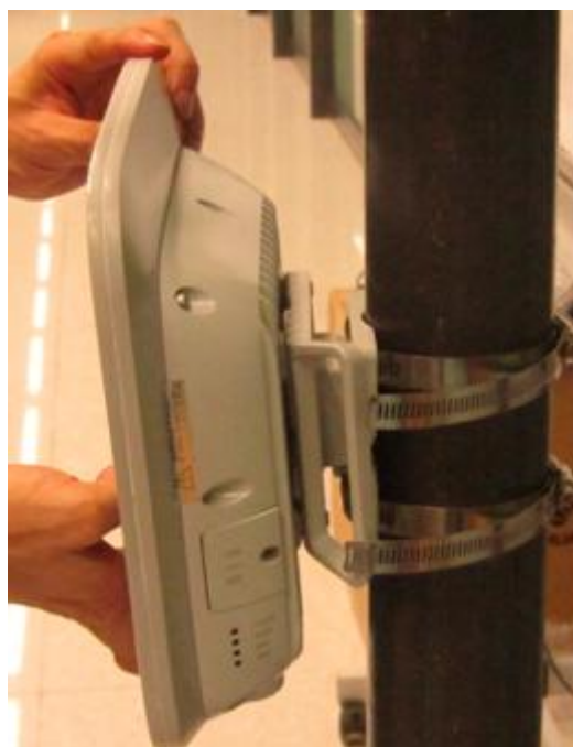
Figure 3-7 Installing the eA680-950 on the wall-mounting frame
