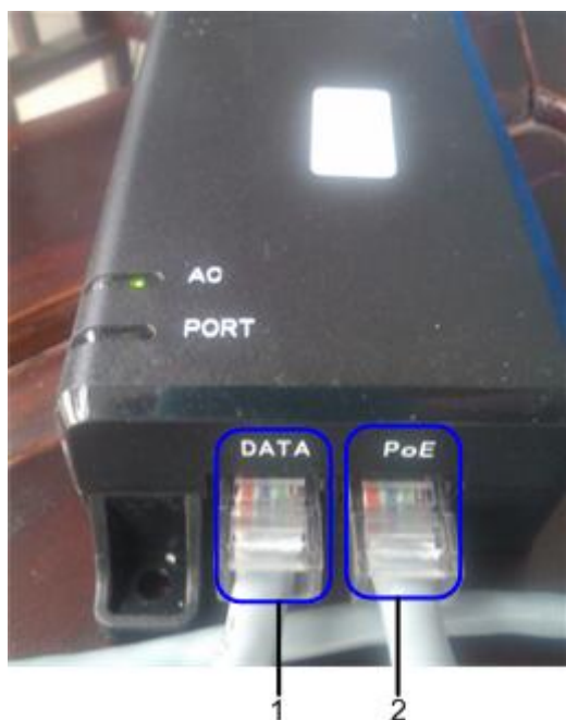
Figure 3-21 Connecting the PoE adapter
