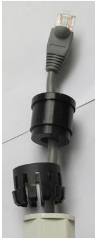
Figure 3-19 Passing the network cable through the PG-head screw cap and air-proof block
