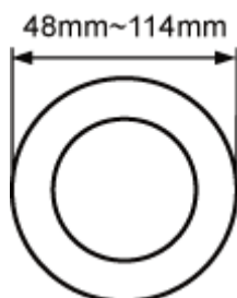
Figure 1-1 Diameter of a pole for installing a eAN3810A
